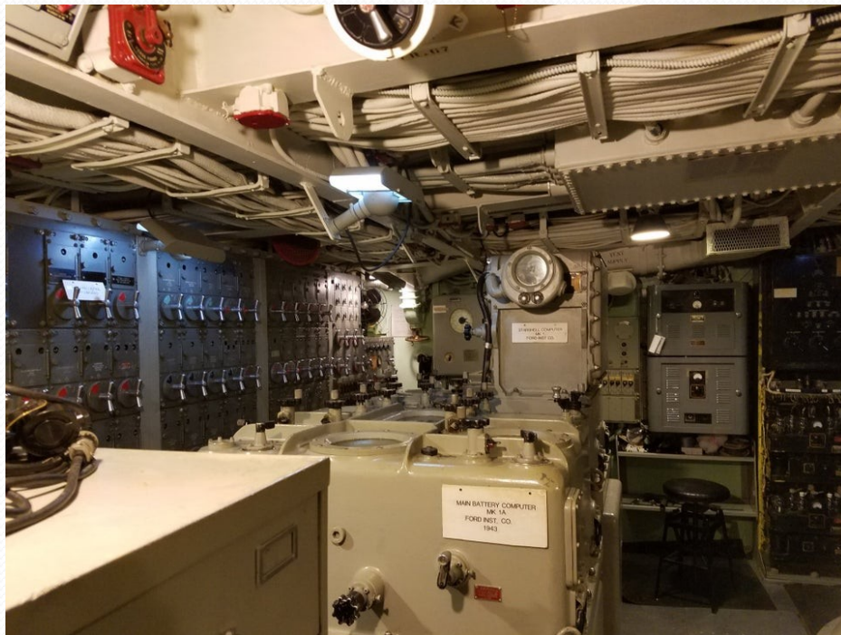
1937 – Mark 1A Fire Control Computer
